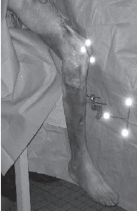
Fig. 2: Experimental Setup showing frames for navigation and axial quadriceps loading.
